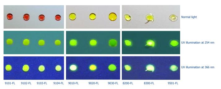
Under UV light, the drop of lubricant emits a green yellow light (around 550 to 600 nm).
